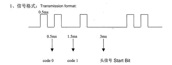
2、**数据包定义:** 每个数据包有 25BIT 数据,如下图所示, Data package: Each data contains 25 bit data, as shown below,
