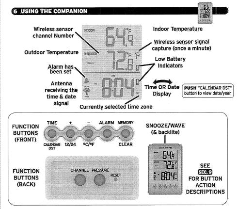
Radio-controlled Clock: The unit starts synchronizing the clock after the 1st channel of the wireless sensor begins to send its information to the main unit. (This is called registration.) The built-in antenna receives the official time signal from the US Government's National Institute of Standards and Technology. A microchip translates the time signal and adjusts the time display for the correct time, and date.
