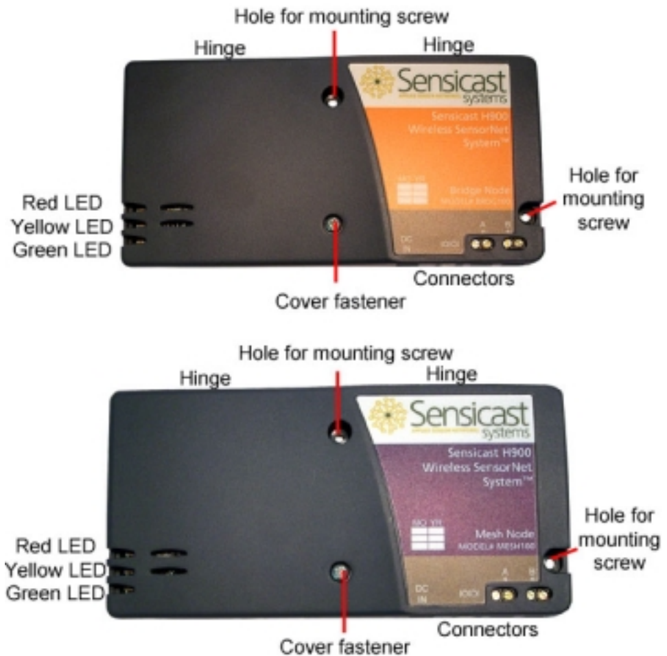
FIGURE 2-1: FRONT OF MESH NODE (PURPLE)/BRIDGE NODE (ORANGE)- COVER CLOSED.
