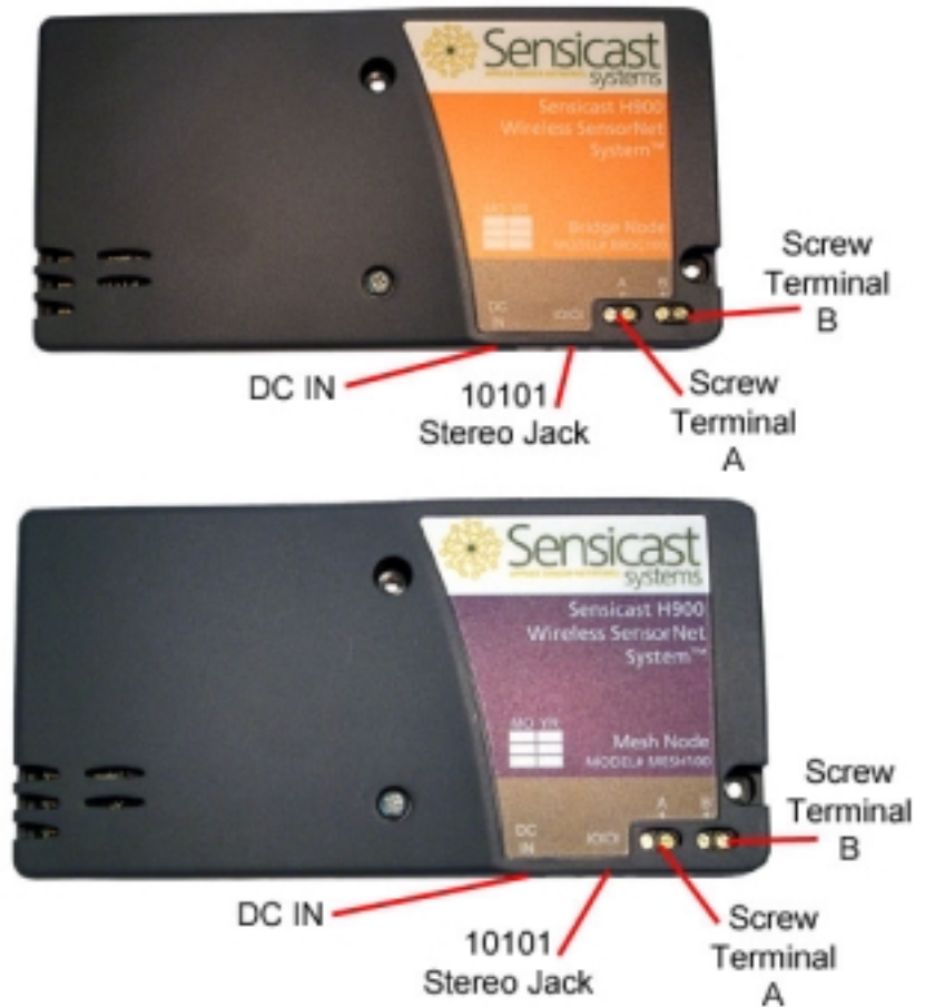
FIGURE 2-5: FRONT OF MESH NODE AND BRIDGE NODE SHOWING EXTERNAL ELECTRICAL INTERFACE.
