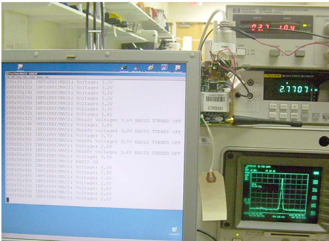
Figure 3.2: Radio turning ON from 3.6V to 3.5V
