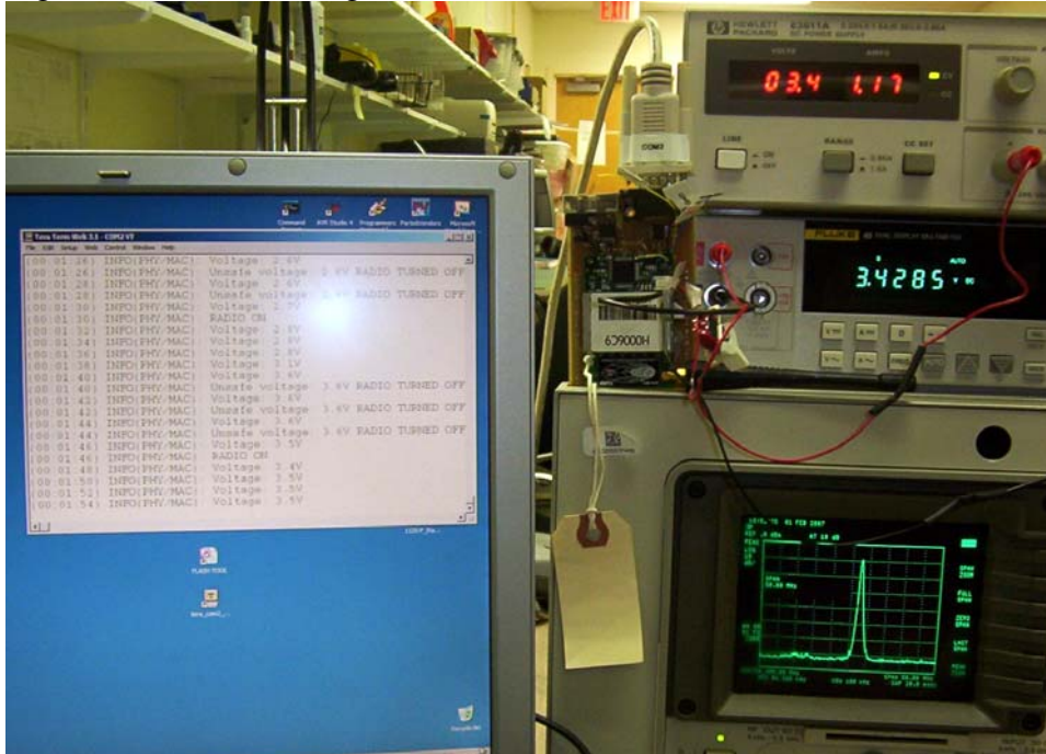
Figure 3.2: Radio turning ON from 3.6V to 3.5V
