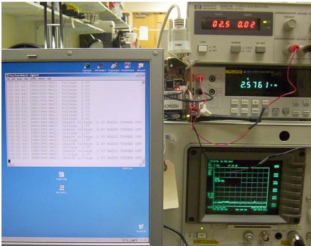
Figure 2.2: Radio turning OFF from 3.2V to 3.8V
