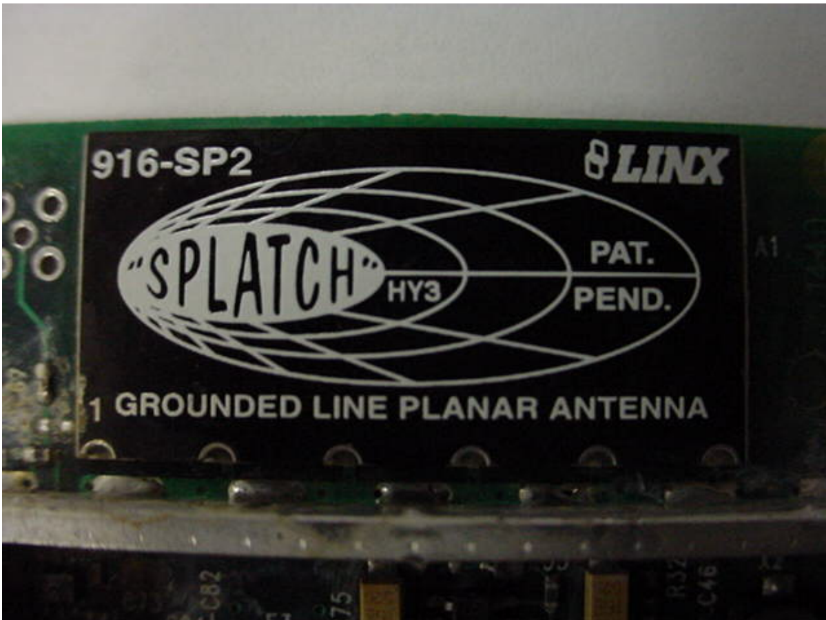
Photo Three – Internal Surface Mount Antenna
