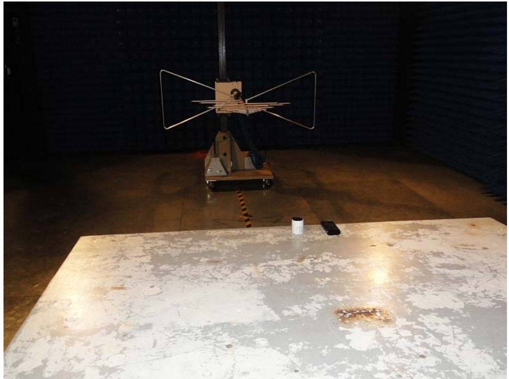
Radiated Emission Test Setup:
