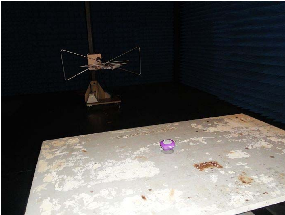
Radiated Emission Test Setup:
