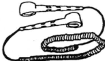
**Flexible cords:** to be connected to the elastic wristband and the special plug on the shelf highlighted with the ESD warning label.
