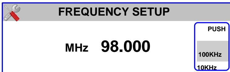
Pressing the rotary switch you can choose the frequency steps between 100 KHz or 10 KHz. Then turning the rotary knob you can reach the desired frequency. Confirmation is done by pressing the rotary encoder for a few seconds.
