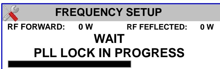
The PLL and ON-AIR LEDs are switched on after the locking time is complete. During the locking time, the traffic light turns yellow and then turns green once the procedure is complete.
