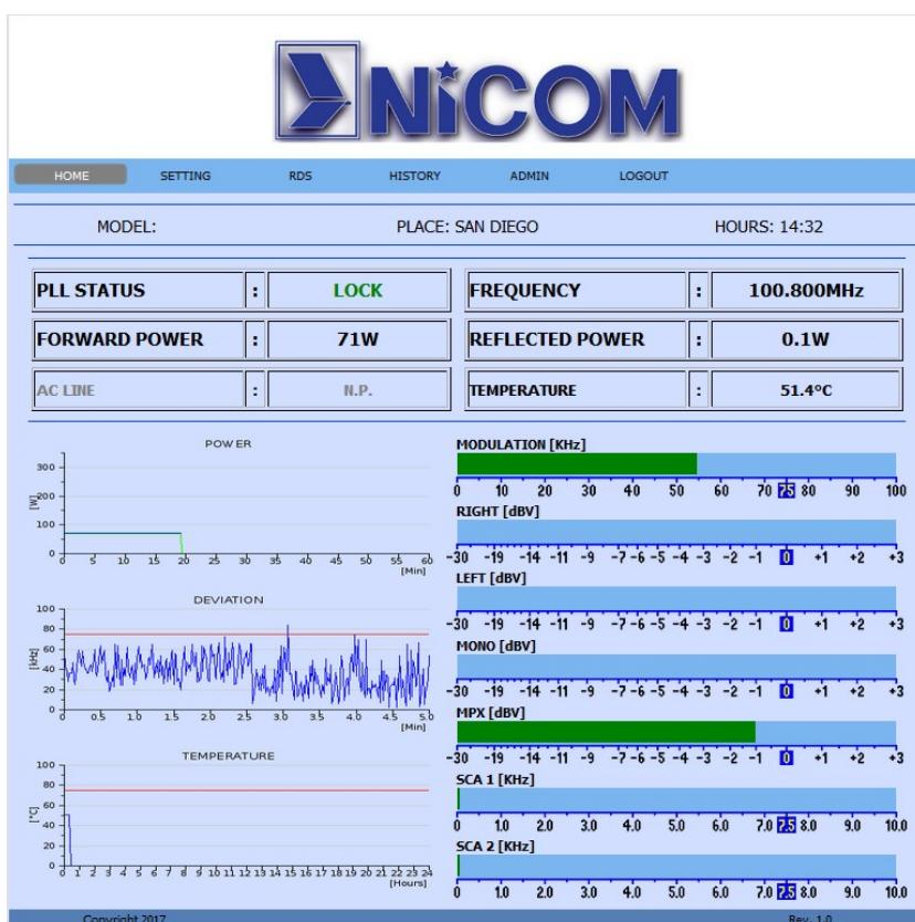
The user Admin has the complete access to the WEB SERVER and its the only one able to set up new users, change settings and allow other users to do so.
