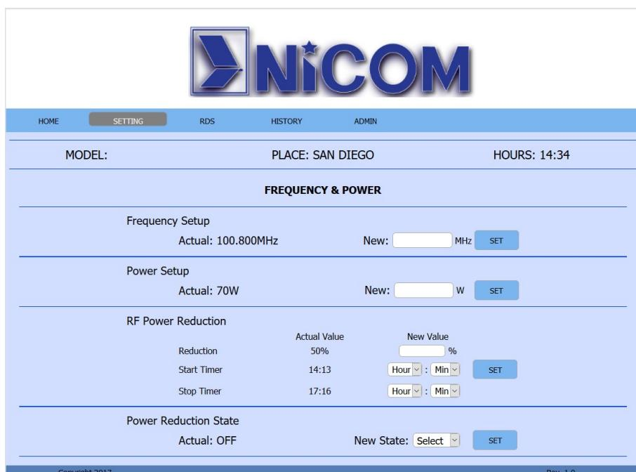
Inside **SETTING** it is also possible to set the Audio Levels in every input of the transmitter. Again all changes needs to be confirmed with the SET button.
