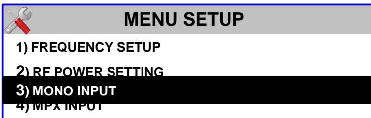
The MONO input is the XLR connector. It is shared with the LEFT input of the STEREO CODER module. By choosing this option you can set some parameters of the MONO input, including the input impedance, pre-emphasis and amplification gain:
