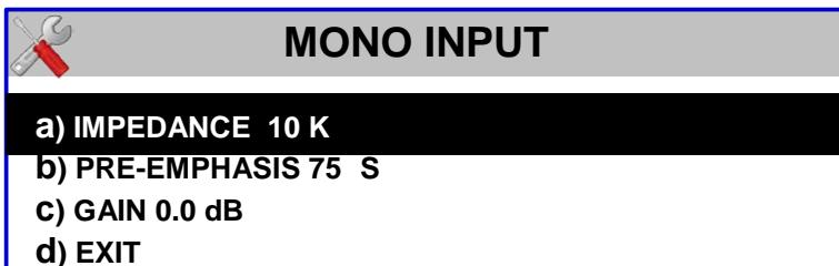
Each access to these parameters gives the possibility of switching from one value to another through the rotary encoder and confirming the choice by pressing it:
