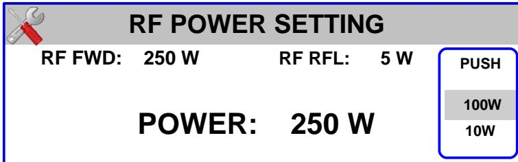
Rotary encoder rotation allows you to increase or decrease the value of the output RF power, short rotary pressure allows you to switch from one movement being 10W to many movements being 100W.
