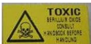
This warning label is used for components containing Beryllium Oxide.
