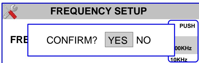
After confirmation, the RF module is turned off processing a new PLL frequency locking;
