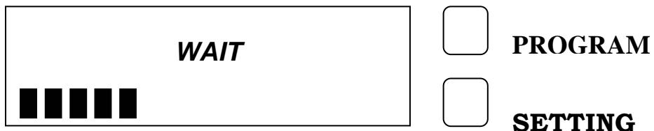
After 3 seconds the green PLL LOCK led will light and the Display will show an increasing bar. After a further 5 seconds the green ENABLE will light and there will be output power.
