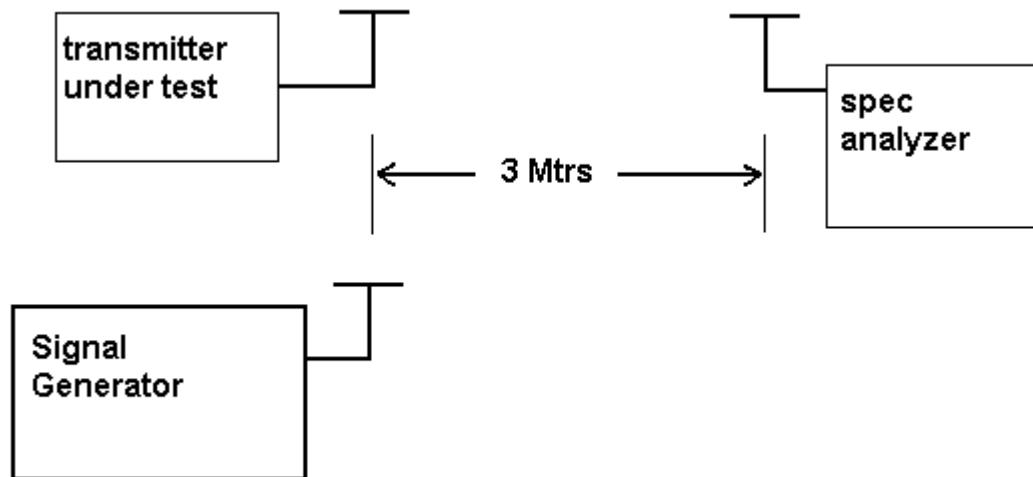
**METHOD OF MEASUREMENT:** The tabulated data shows the results of the radiated field strength emissions test. The spectrum was scanned from 30 to at least the tenth harmonic of the fundamental. This test was conducted per ANSI/TIA-603-C-2004 using the substitution method. Measurements were made at the open field test site of TIMCO ENGINEERING, INC. located at 849 N.W. State Road 45, Newberry, FL 32669.
