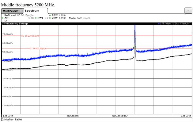
The peak above the limit is the carrier frequency. This plot is valid for Chain A, Chain B, Chain A+B.
