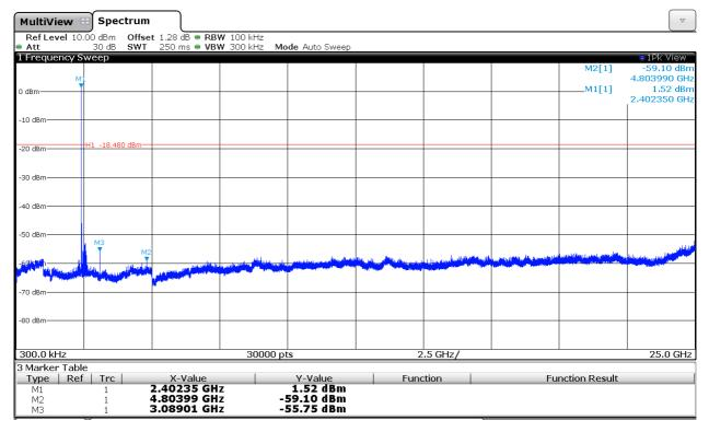
Note: The peak above the limits is the carrier frequency.
