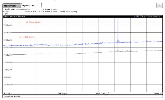
Note: The peak shown in the plot is the carrier frequency.
