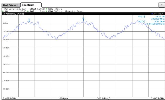
The hopping channel carrier frequencies are separated by a minimum of the 20 dB bandwidth of the hopping channel.
