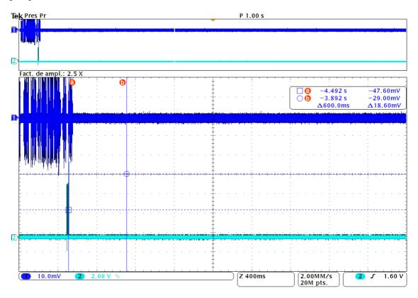
This plot provides a zoom-in to show the 600 ms time interval after the radar burst. This shows that there were not any transmissions after 200 ms following the radar burst.
