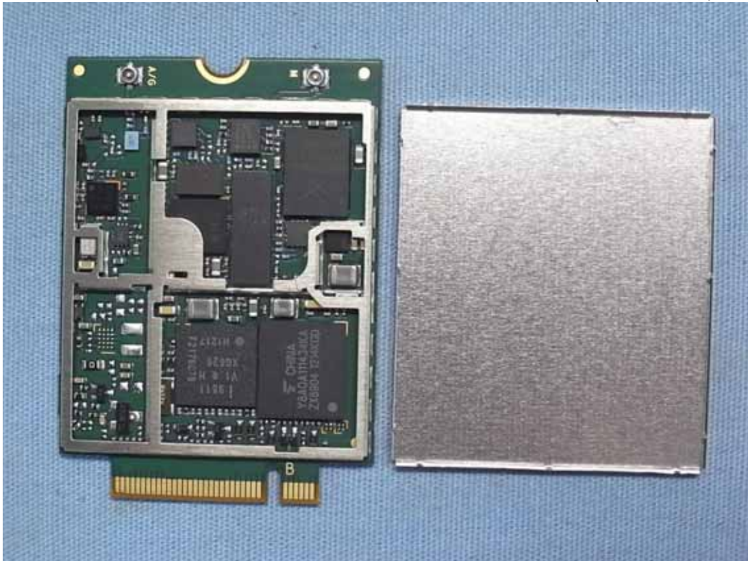
Figure 21 Internal View (3G Module, Front View)
