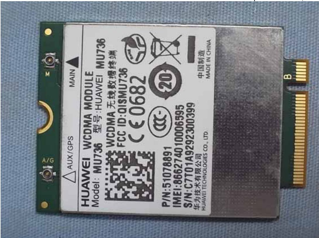
Figure 20 Internal View (3G Module, Front View)
