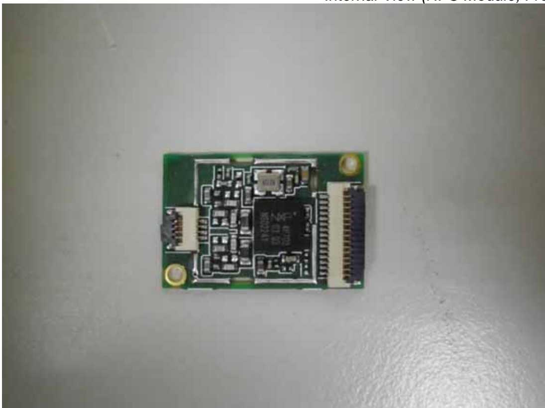
Figure 36 Internal View (NFC Module, Front View)
