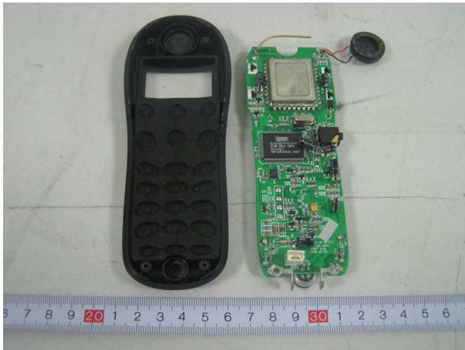
EUT- Handset inside View (2)
