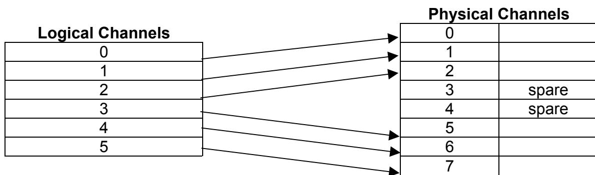
Noisy channels can be adapted out of the sequence by 'channel swapping', *i.e.* swapping a good spare channel for a noisy channel. For example, swapping physical channels 1 and 3 gives:
