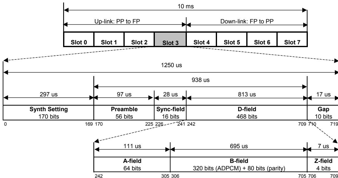
The basic, repeating, frame structure is 10 ms long. It is sub-divided into 8 slots, each 1250  $\mu$ s long. The active transmission time is 937.5  $\mu$ s. The first 4 slots form the 'up-link', when the PPs transmit to the FP. The last 4 slots form the 'down-link', when the FP transmits to the PPs.
