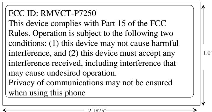
**Specifications:** Text is black or white in color and is left justified. Labels are silk-screened and shall be “permanently affixed” at a conspicuous location on the EUT.
