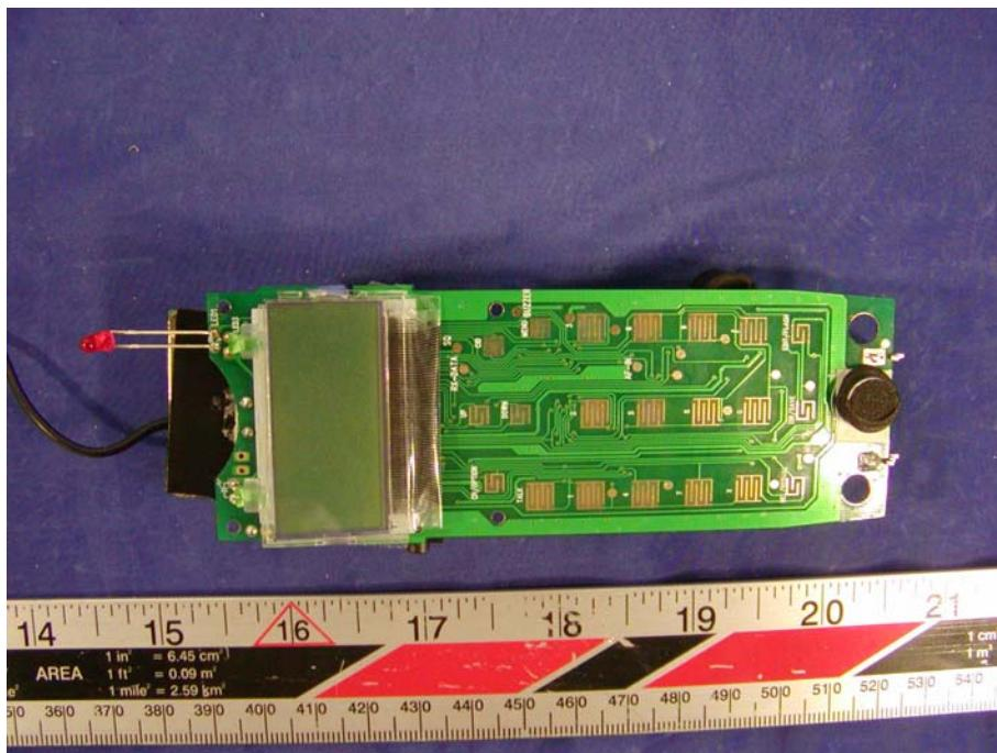
**Handset transceiver solder view**
