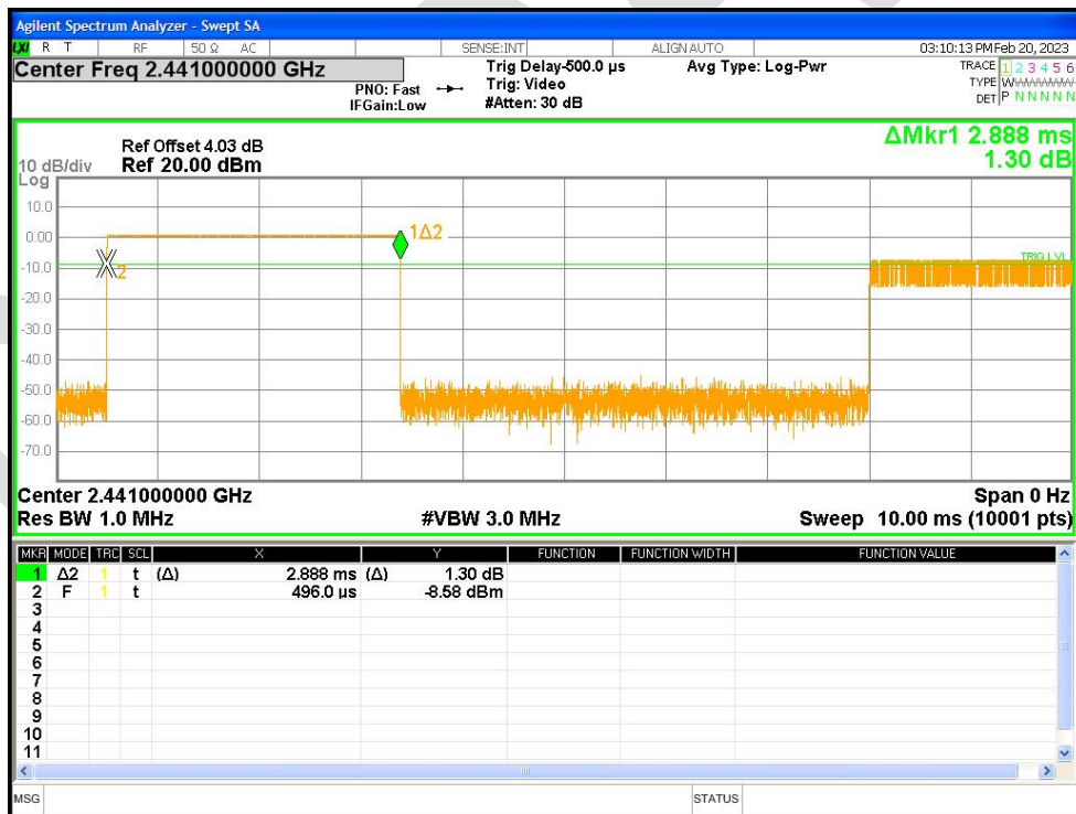
Dwell NVNT 1-DH5 2441MHz Ant1 Accumulated
