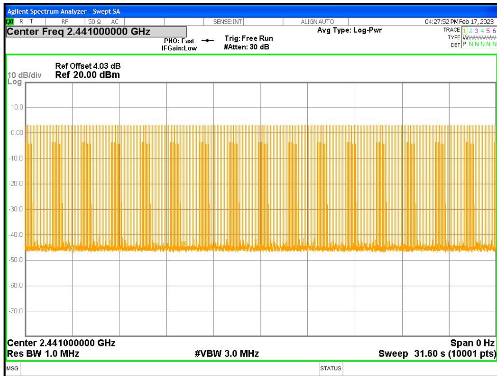
Dwell NVNT 3-DH5 2441MHz Ant1 One Burst
