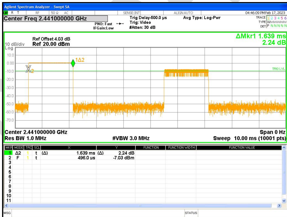
Dwell NVNT 1-DH3 2441MHz Ant1 Accumulated
