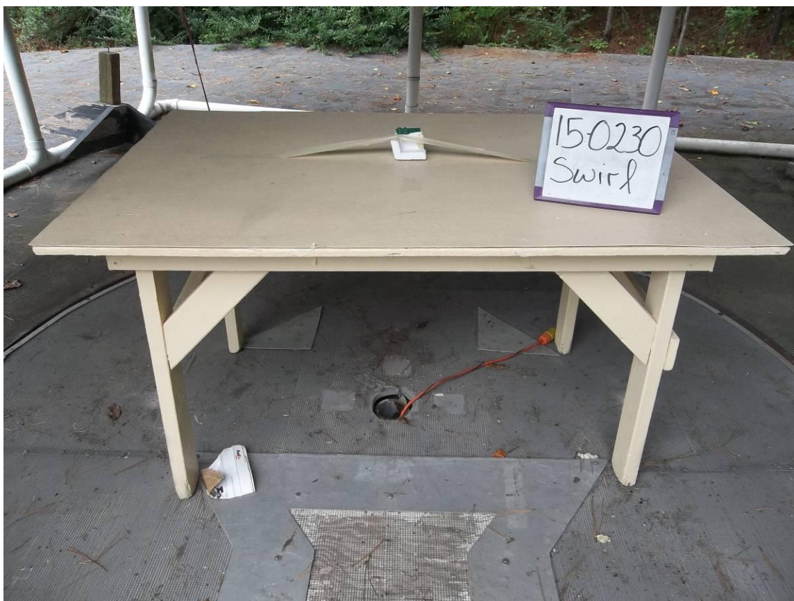
Figure 1. Radiated Emissions Test Configuration, Front
