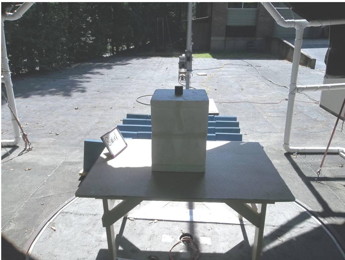
Figure 7. Radiated Emissions Test configuration, Intentional Emissions above 1 GHz
