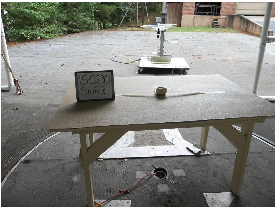
Figure 4. Radiated Emissions Test Configuration, 200-1000 MHz
