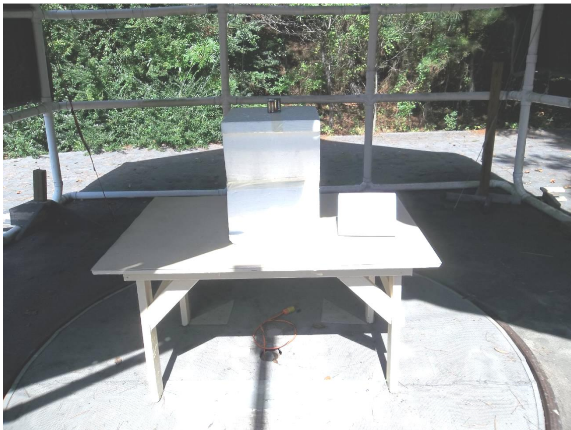
Figure 6. Radiated Emissions Test Configuration, Intentional Emissions above 1 GHz (Front)
