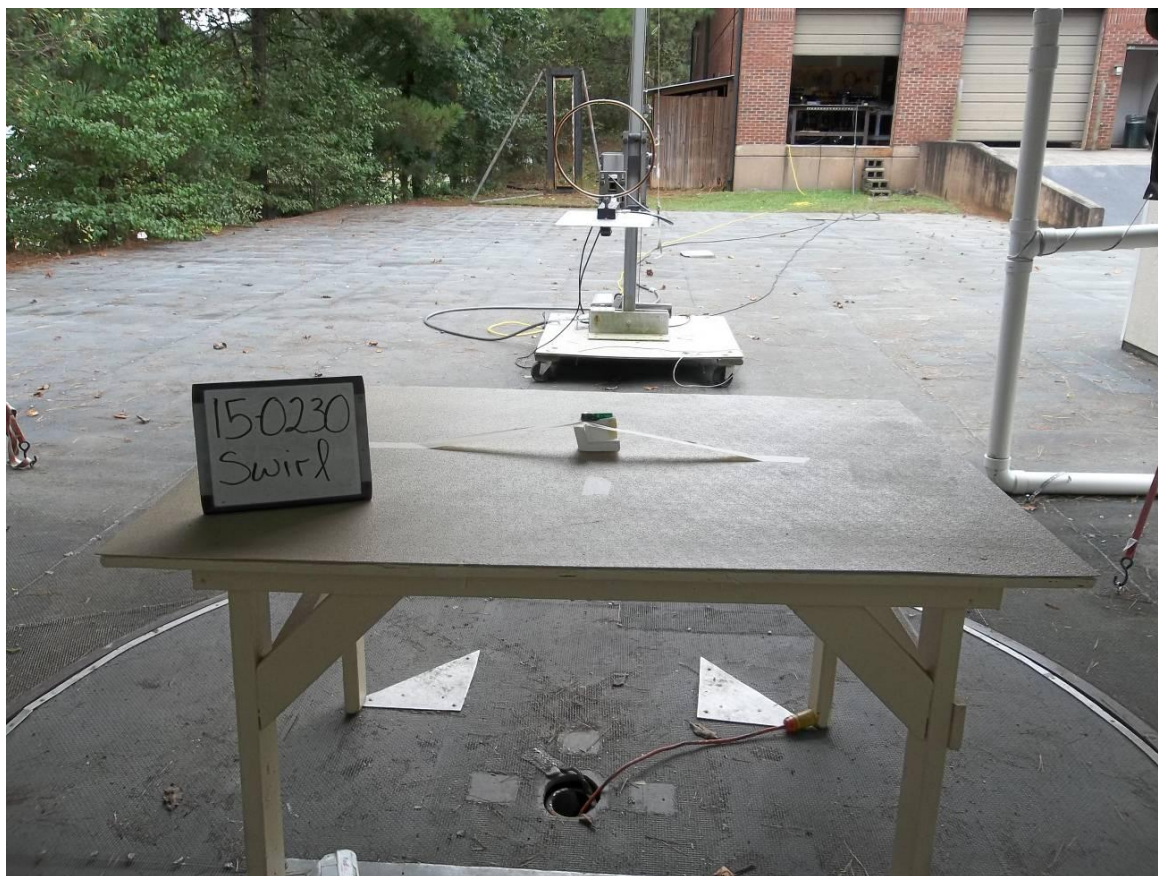
Figure 2. Radiated Emissions Test Configuration, Below 30 MHz
