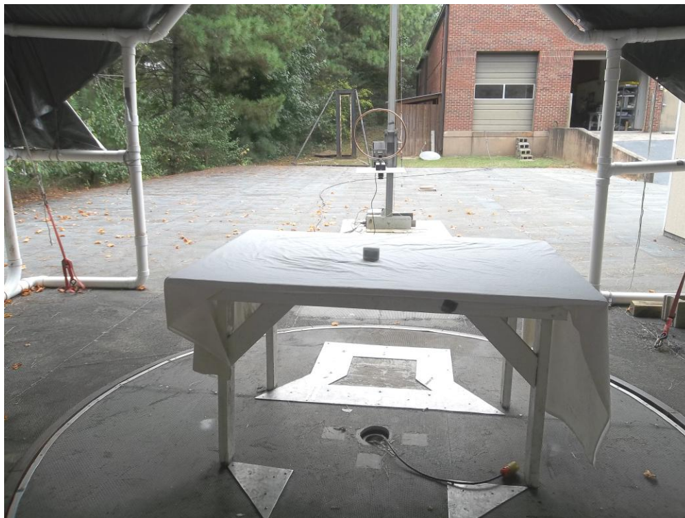
Figure 3. Radiated Emissions Test Setup - Below 30 MHz
