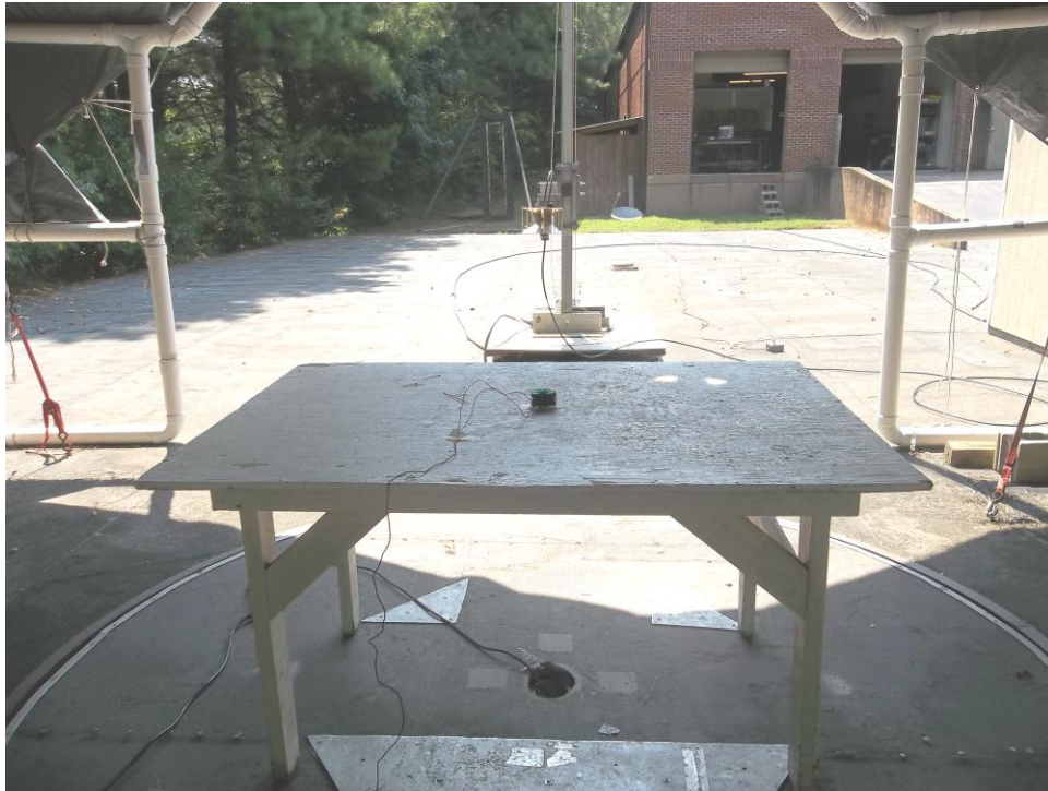
Figure 6. Radiated Emissions Test Setup - above 1000 MHz
