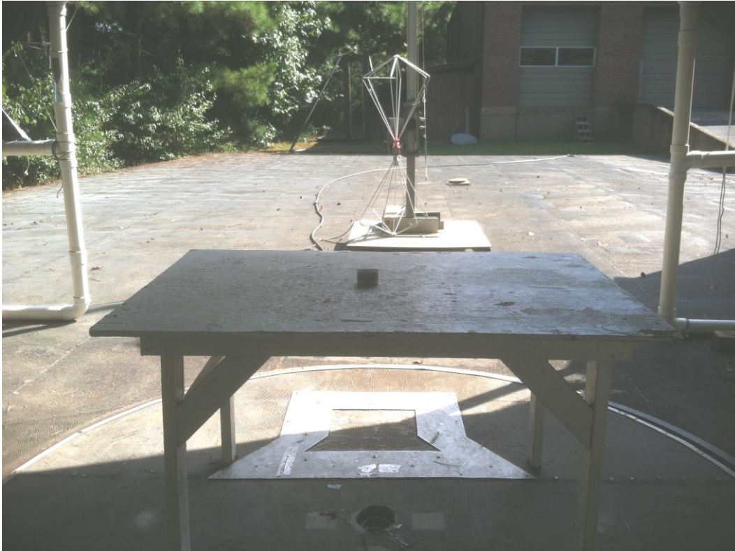
Figure 4. Radiated Emissions Test Setup - 30-200 MHz
