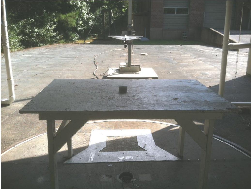
Figure 5. Radiated Emissions Test Setup - 200-1000 MHz
