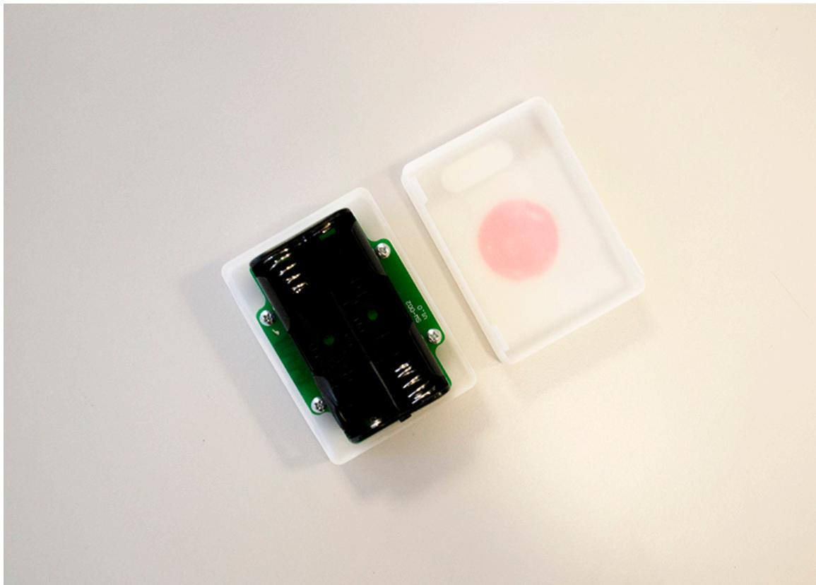
3. Place the two provided AA batteries in the battery holder making sure to align the positive (+) and negative (-) terminals of the battery as indicated by the diagram markings inside the holder.
