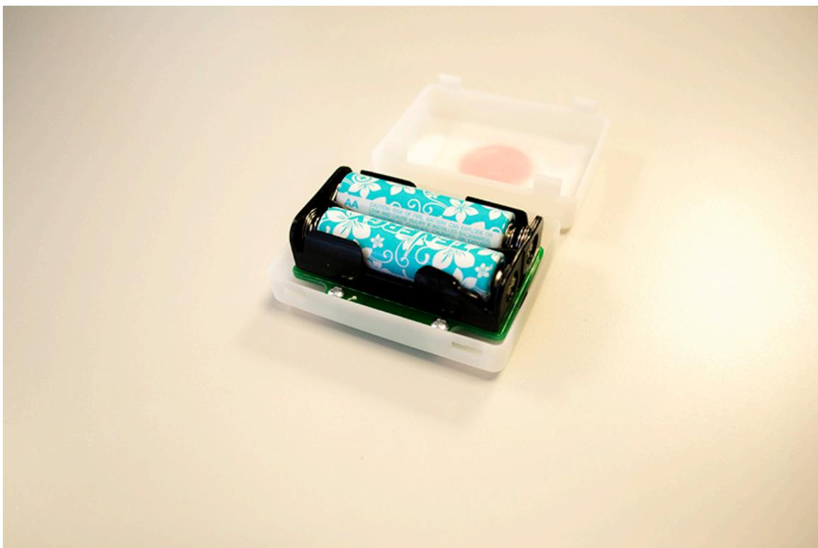
4. Re-assemble the top and bottom cases by aligning the two sections over one another while squeezing the sides of the bottom case allowing the bottom case tabs to clear the inside of the top case and snap into place.
