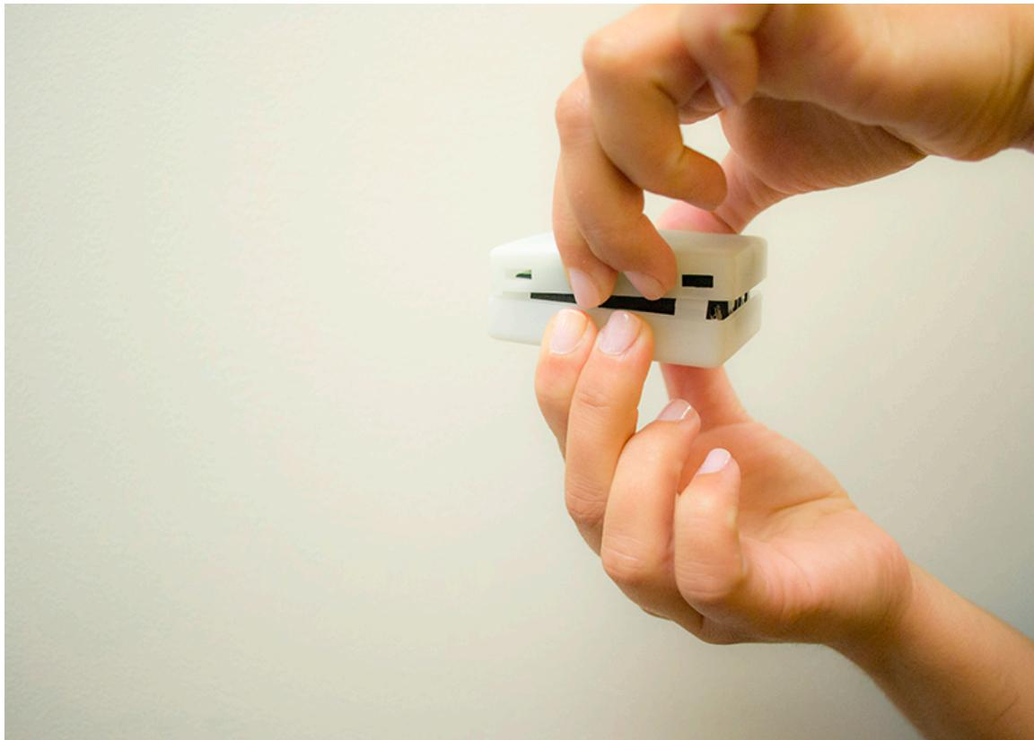
2. Turn the top section of the case upside down to reveal the enclosed circuit board and plastic battery holder.
