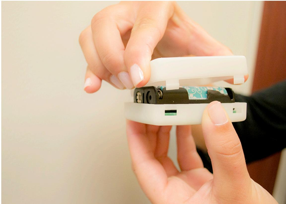
5. Once the battery is properly installed, the Swirl Sensor will automatically start broadcasting and advertising its presence. The sensor will automatically be placed into a continuous broadcasting state until the battery is either removed or is depleted of its power.
