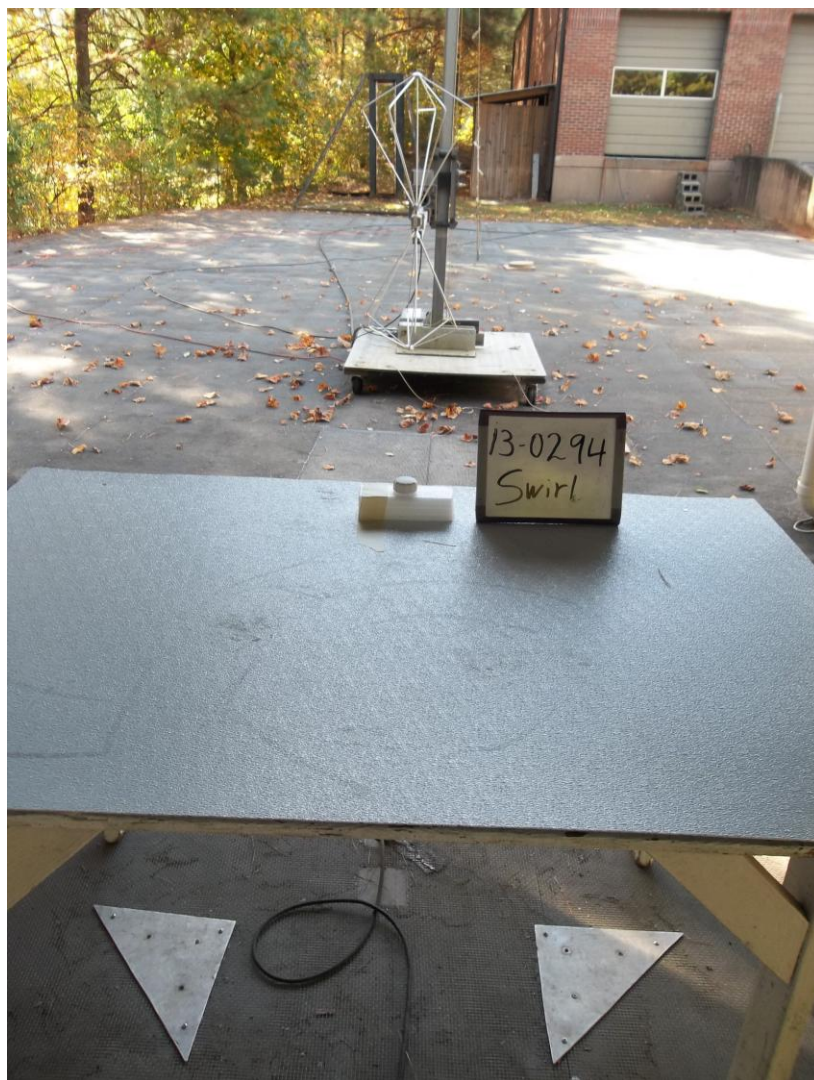
Figure 3. Radiated Emissions Test Setup - 30-200 MHz
