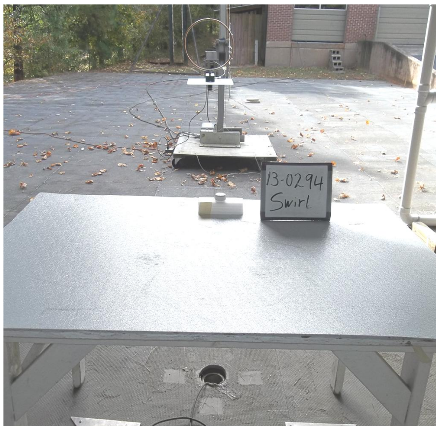
Figure 2. Radiated Emissions Test Setup - Below 30 MHz
