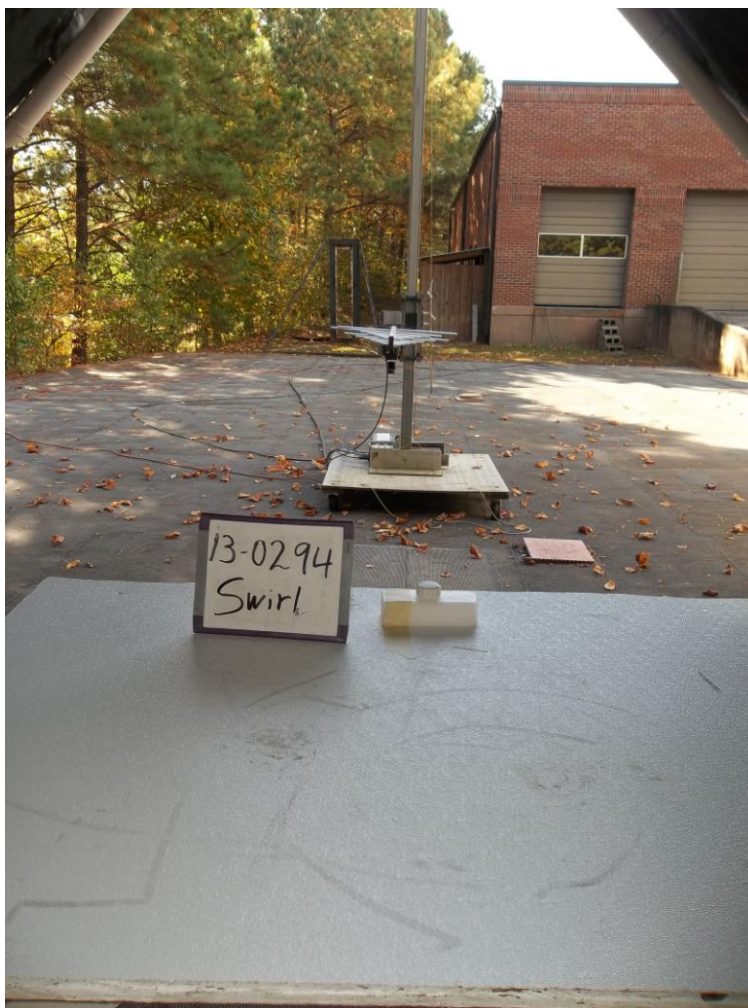
Figure 4. Radiated Emissions Test Setup - 200-1000 MHz
