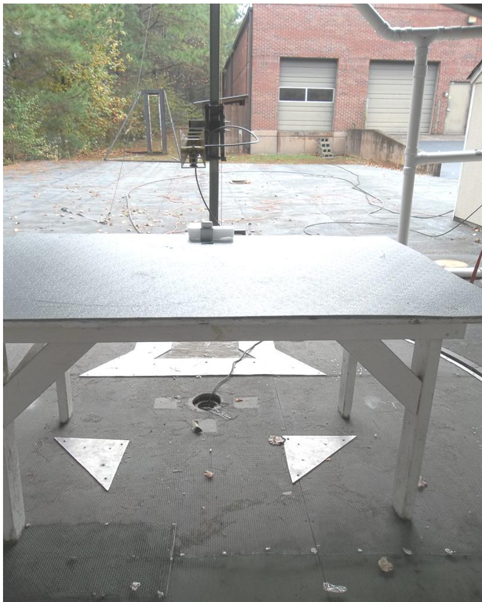
Figure 5. Radiated Emissions Test Setup - above 1000 MHz
