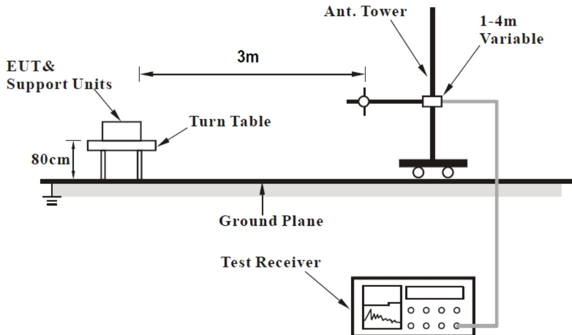
(B) Radiated Emission Test Set-Up, Frequency above 1000 MHz
