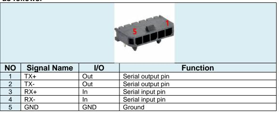
Power (43650-0200): Arrangement of connectors to connect with the exclusive adaptor, used connectors and pins would be as follows.
