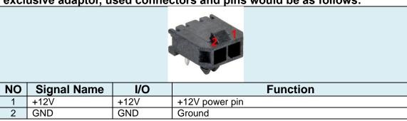
CID Checker (55959-0830): This is a connector to connect with the external device to check if it operates correctly by supplying the power to CID-R. Arrangement of used connectors and pins would be as follows.
