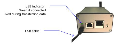
The maximum length for a USB connection is limited to 5 meters.
