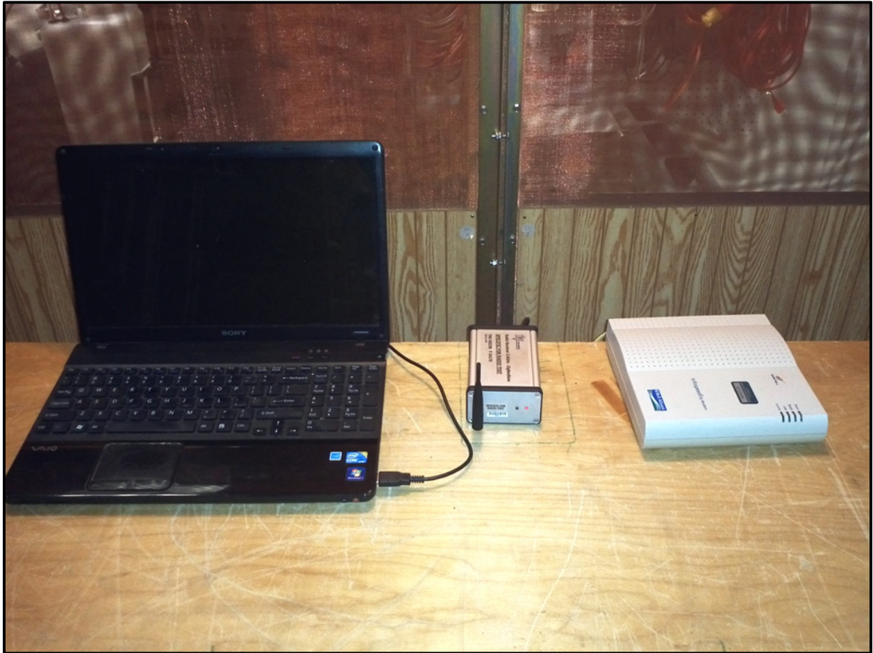
Photograph 5: AC Conducted Testing – Front View – AC Adapter
