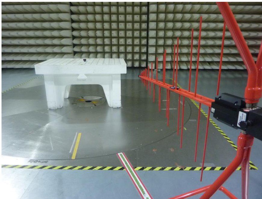
Figure 2: Test Setup for 30 MHz to 1 GHz (Front View)
