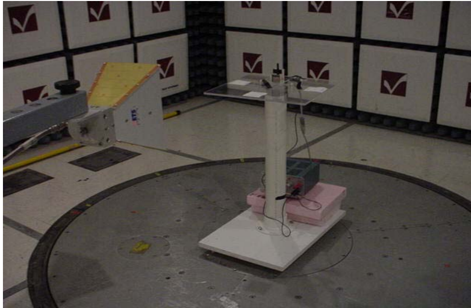
View of the EUT during Radiated Emission Testing in the 3 Meter FCC Listed Chamber, Antenna A
