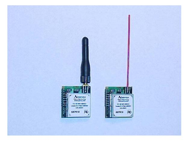
ALERTx Transceiver Module 902 to 928 MHz Digital Radio
