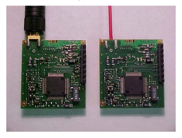
ALERTx Transceiver Module 902 to 928 MHz Digital Radio
