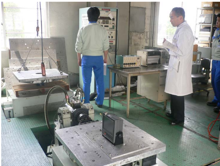
Figure 6-7 EUT in Axis-X Vibration Test, 24th May, 10:26
