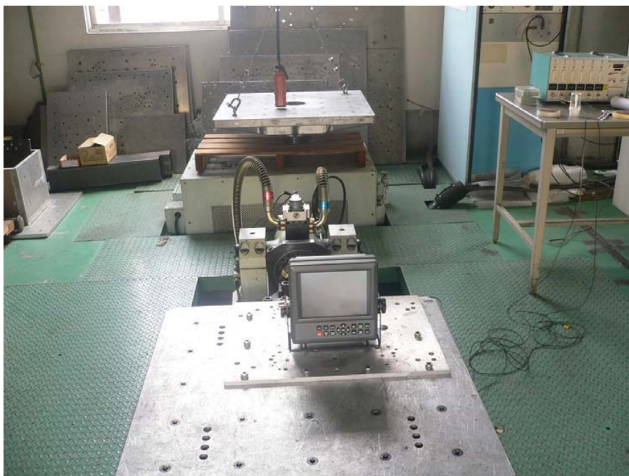
Figure 6-8 EUT in Axis-Y Vibration Test, 24th May, 13:50
