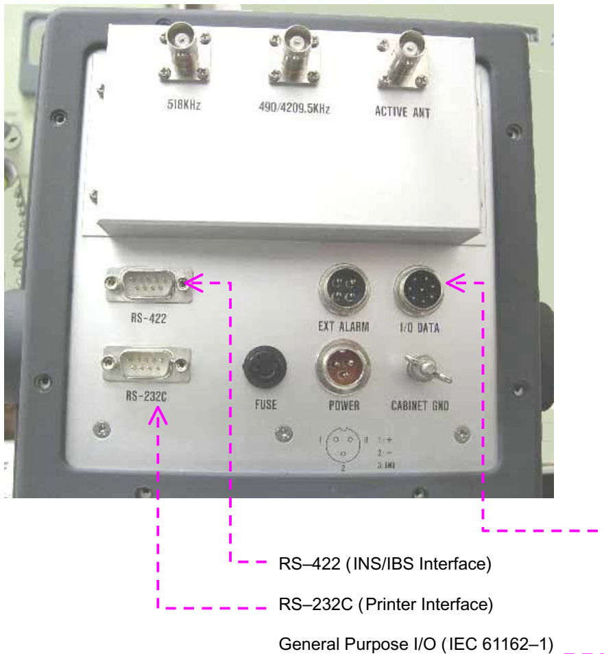
Figure 17 Rear Panel Digital Interface Connectors [as per MSC.148(77) Annex 10, paragraphs 9.1 through 9.3]
