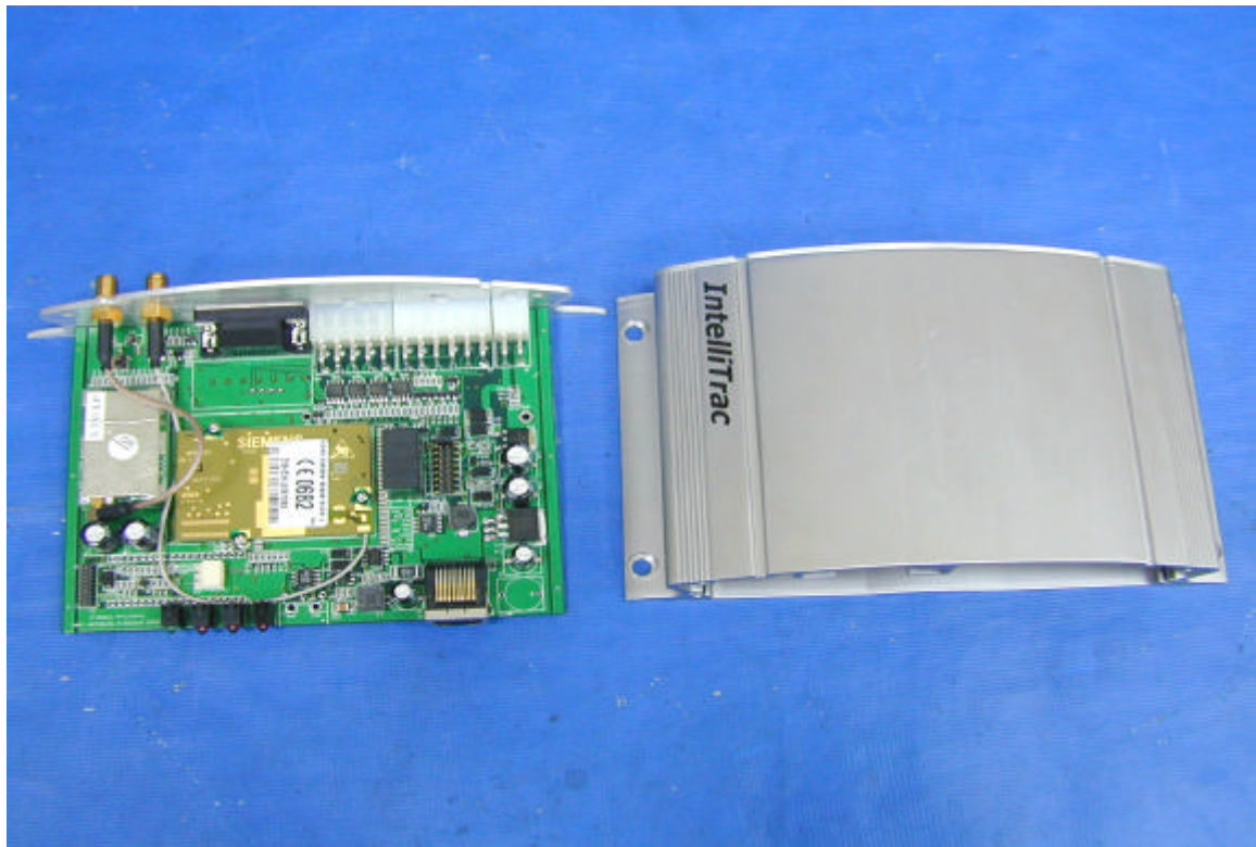
PHOTO. 3. EUT INSIDE VIEW
