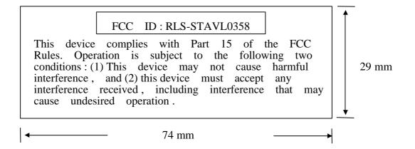
The modular transmitter must be labeled with its own FCC ID number, and, if the FCC ID is not visible when the module is installed inside another device, then the outside of the device into which the module is installed must also display a label referring to the enclosed module:
