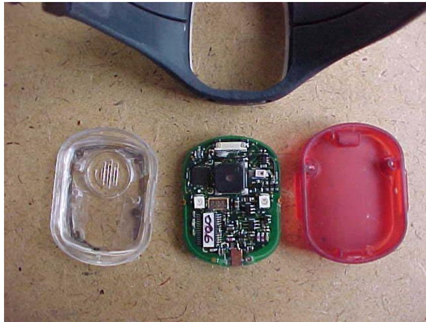
**Internal View of EUT with Battery Removed**
