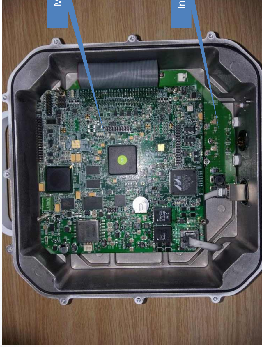
Photo of ODU showing services compartment with rear cover removed
