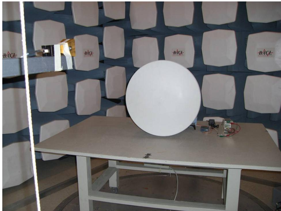
**13.12 (20 GHz – 140 GHz) Radiated Emission 24 inches Antenna – Rear View**
