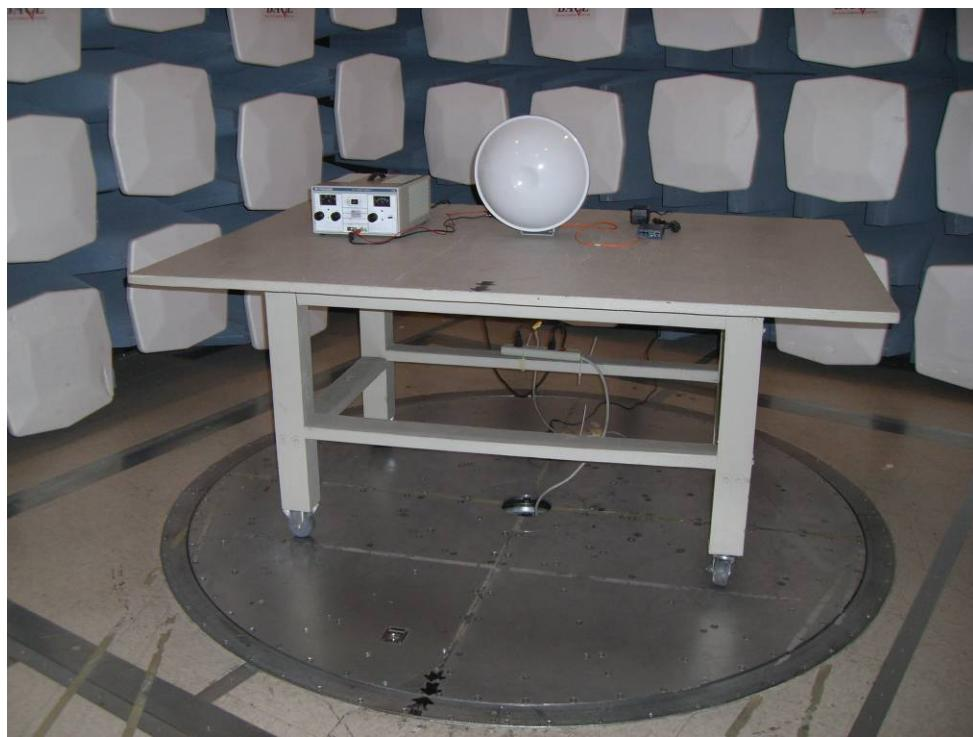
**13.6 (30 MHz - 1GHz) Radiated Emission 12 inches Antenna – Rear View**
