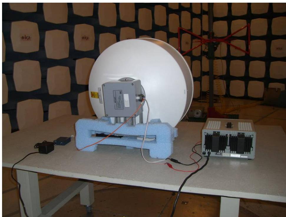
**13.5 (30 MHz - 1GHz) Radiated Emission 12 inches Antenna – Front View**
