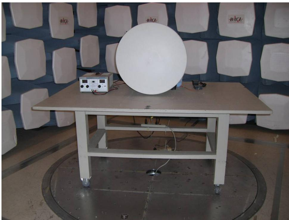
**13.4 (30 MHz - 1GHz) Radiated Emission 24 inches Antenna – Rear View**
