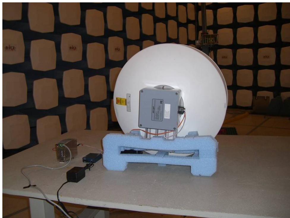
**13.9 (1 GHz – 20 GHz) Radiated Emission 12 inches Antenna – Front View**
