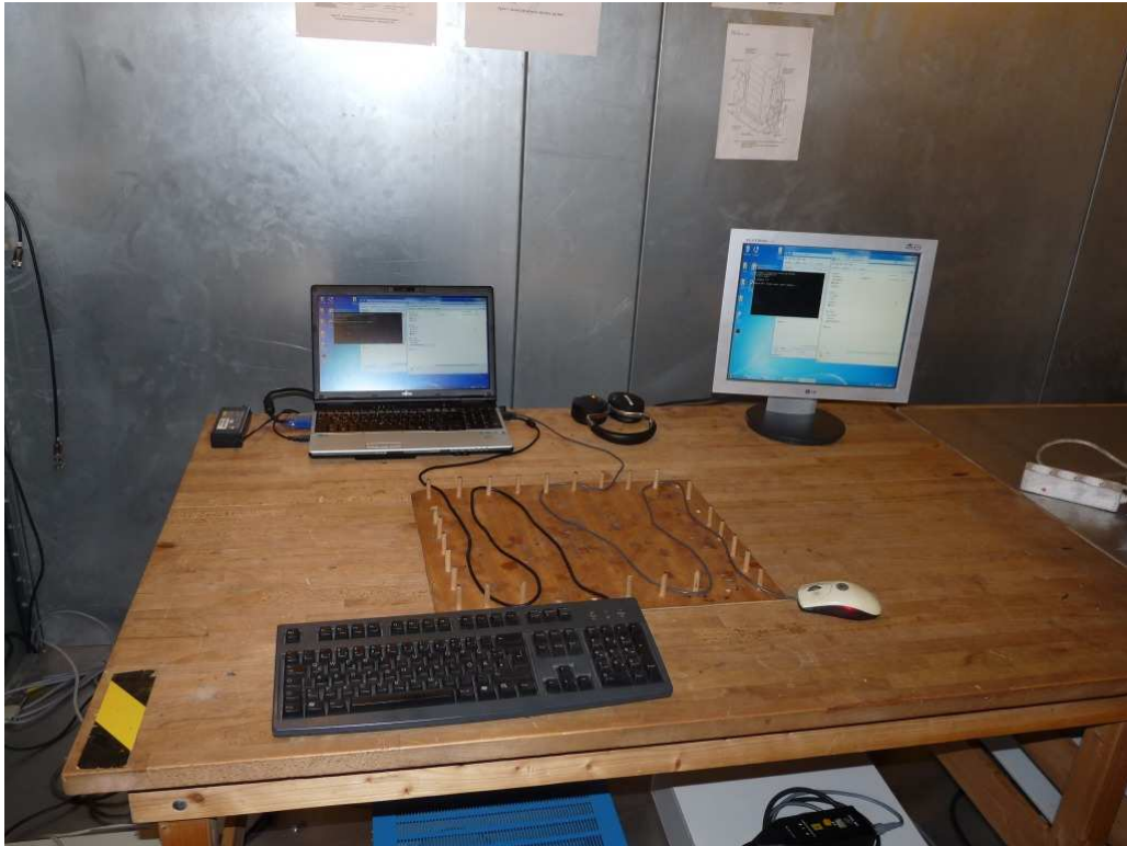
Photo 4: Test setup for conducted measurements, AC Mains
