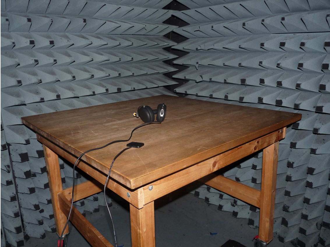
Photo 1: Test setup for radiated measurements (below 30 MHz)
