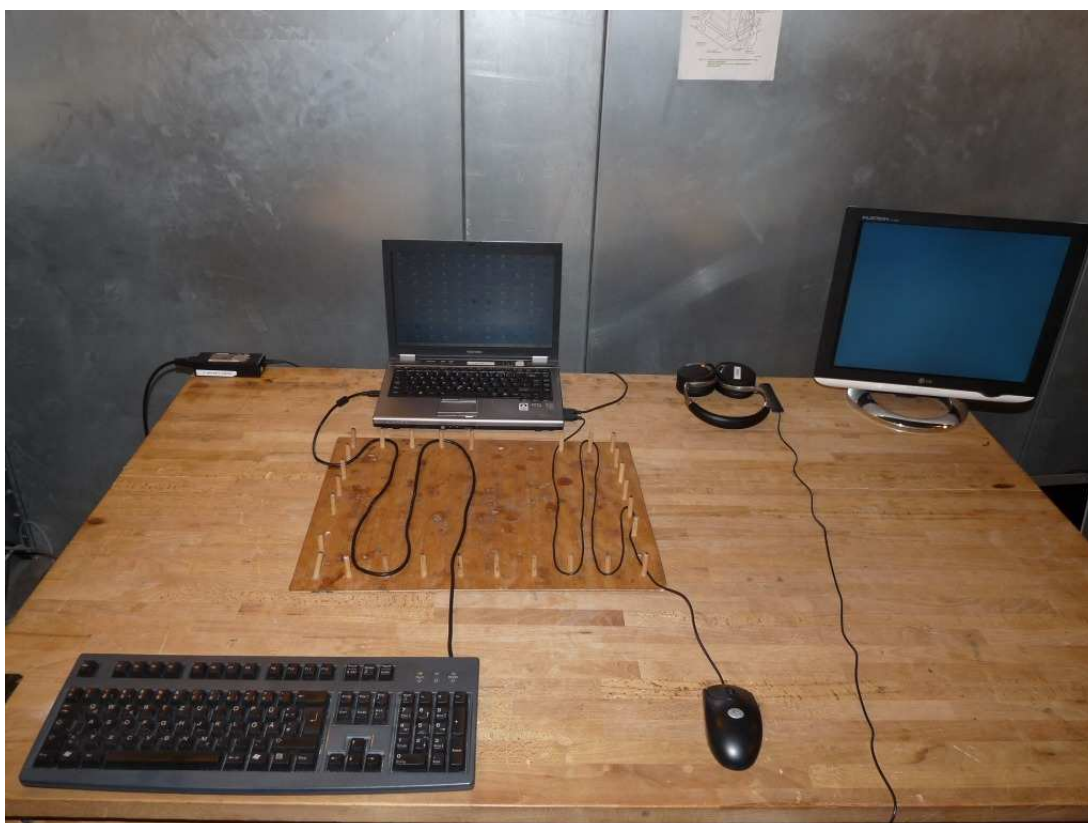
Photo 5: Test setup for conducted measurements, AC Mains
