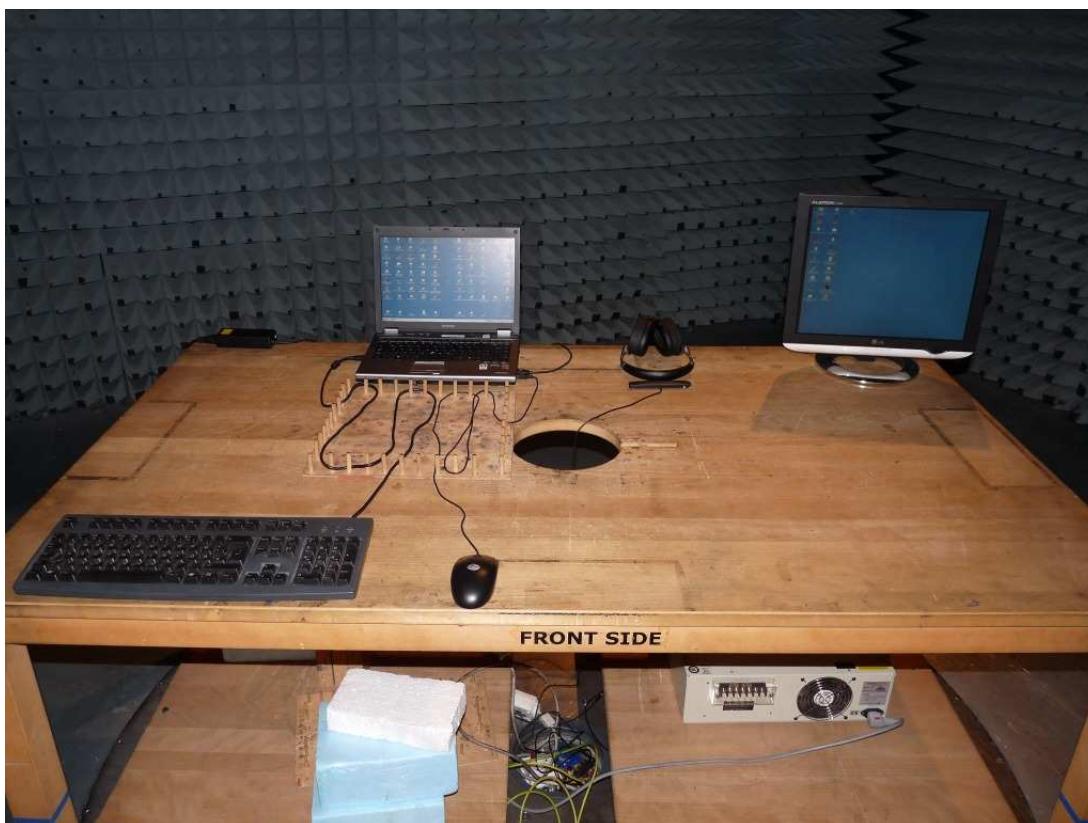
Photo 4: Test setup for radiated measurements (30 MHz to 1 GHz), FCC 15b: Computer peripheral setup
