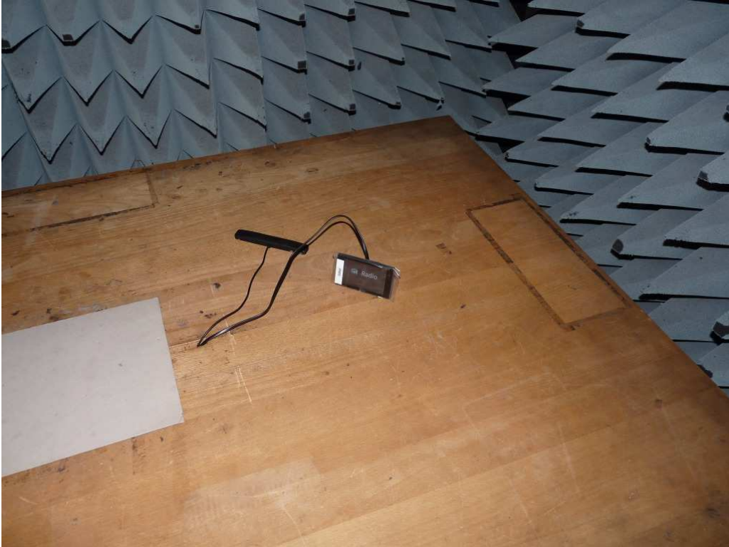
Photo 1: Test setup for radiated measurements (below 30 MHz)
