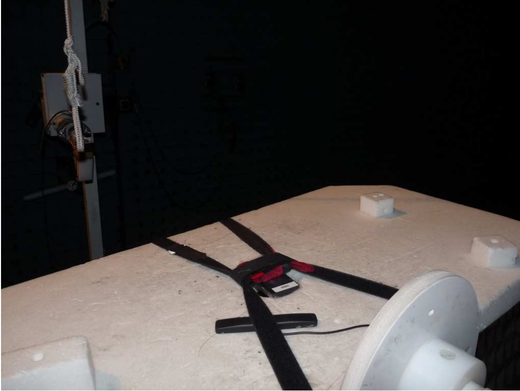
Photo 4: Test setup for radiated measurements (above 1 GHz)
