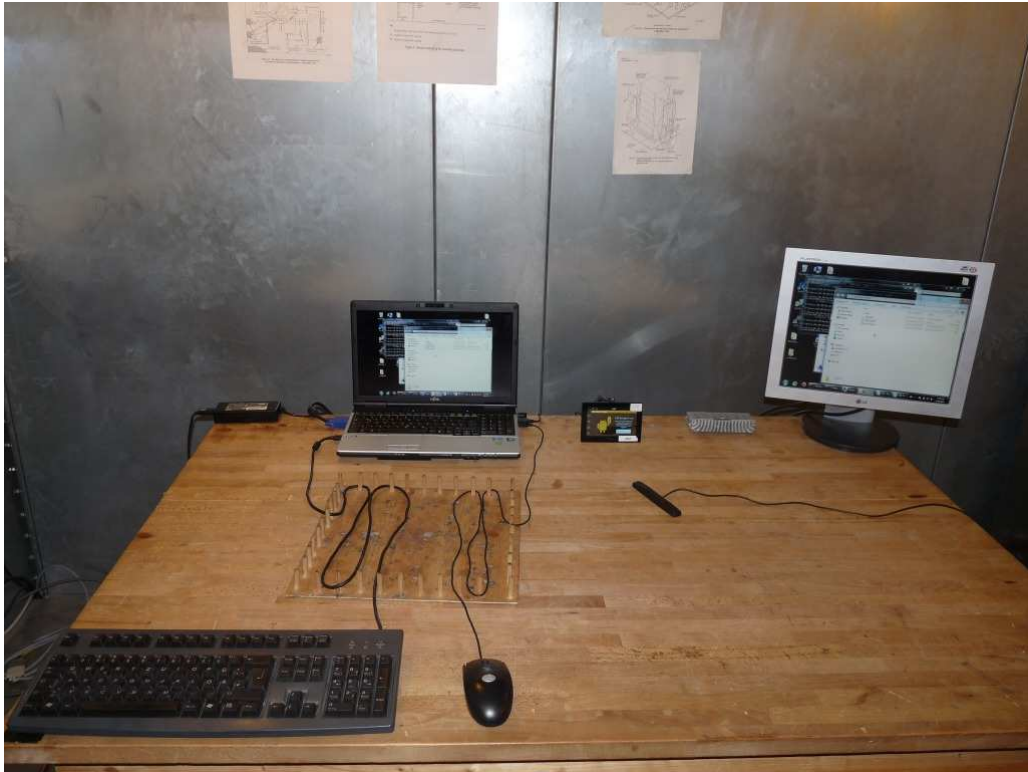
Photo 4: Test setup for conducted measurements, AC Mains
