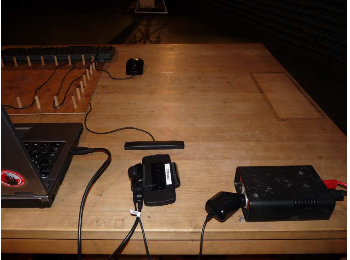
Test Setup Photo: radiated measurements
