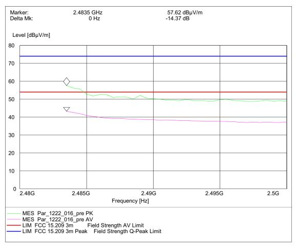
Radiated measurement (higher band edge)
