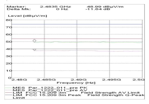
Radiated measurement (higher band edge)
