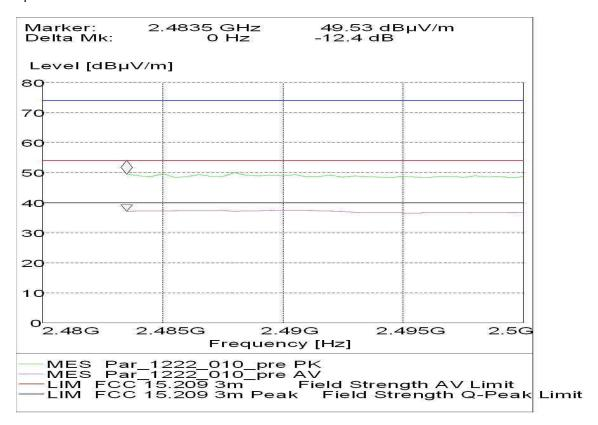
Radiated measurement (higher band edge)
