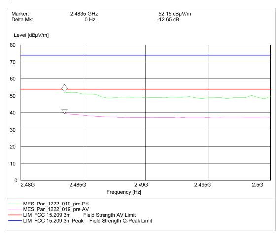
Radiated measurement (higher band edge)
