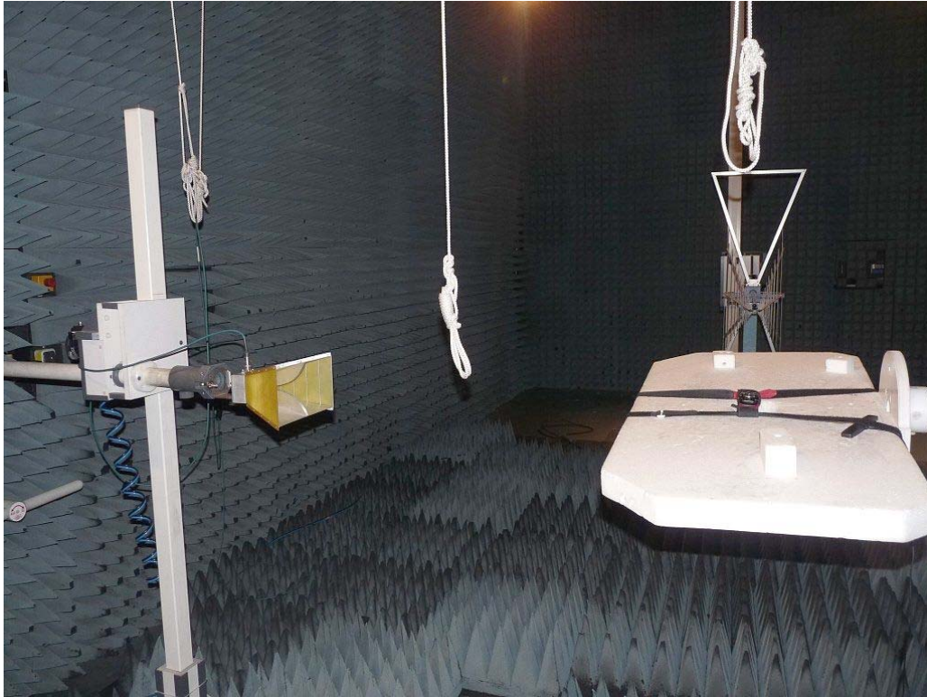
Photo 3: Test setup for radiated measurements, above 1 GHz
