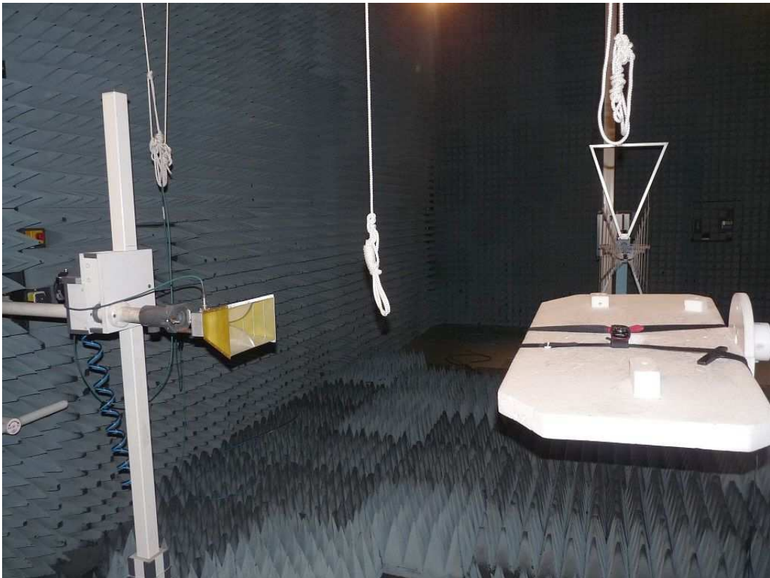
Photo 3: Test setup for radiated measurements (above 1 GHz)
