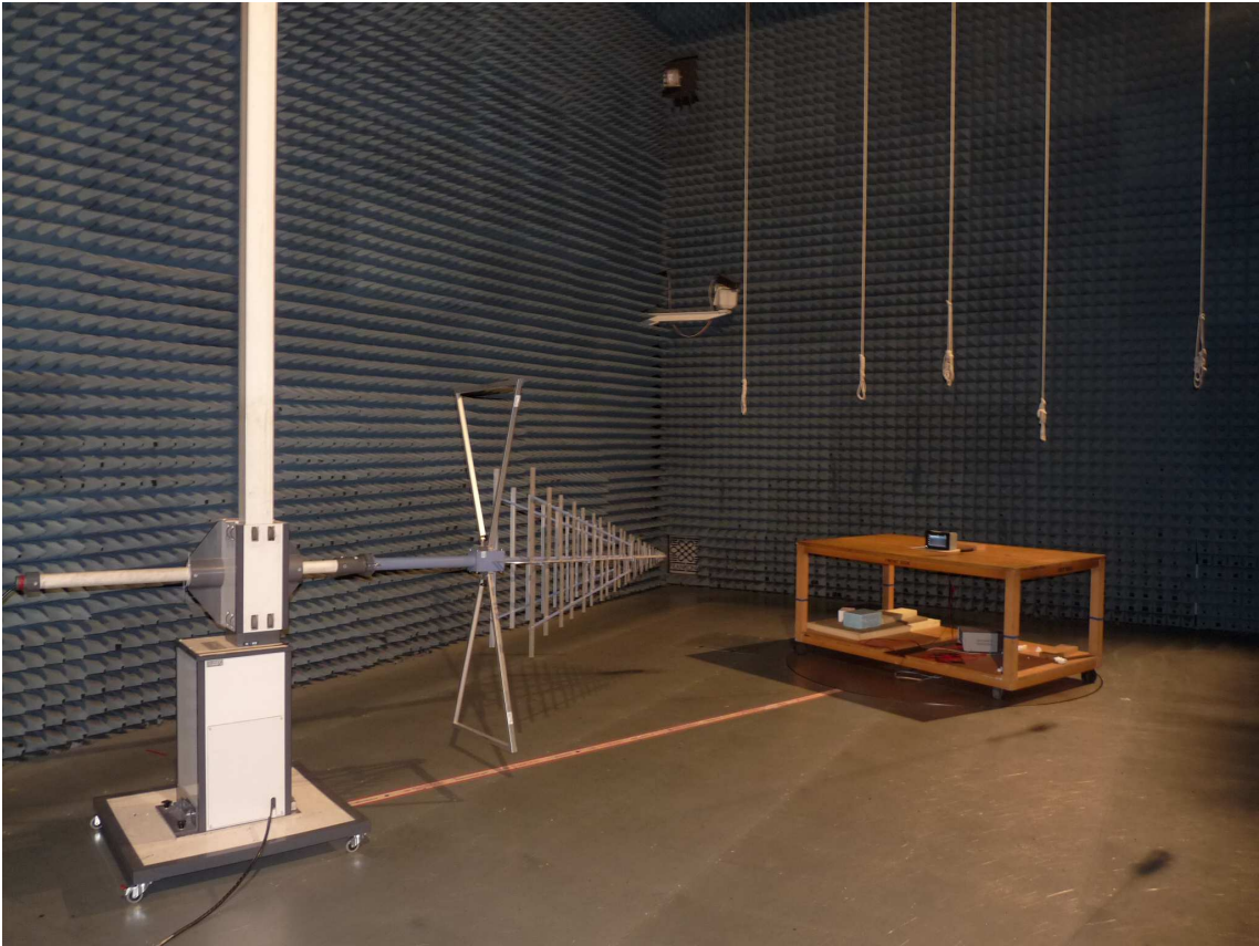
Photo 2: Test setup for radiated measurements (30 MHz to 1 GHz), FCC 15.247
