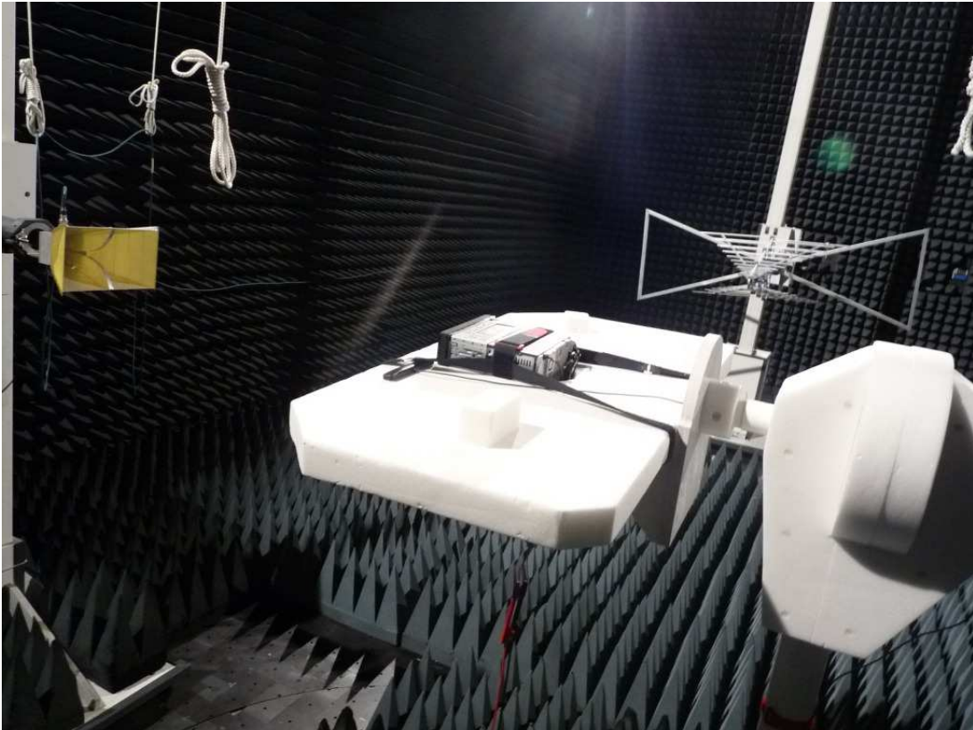
Photo 3: Test setup for radiated measurements (Enclosure, above 1 GHz)
