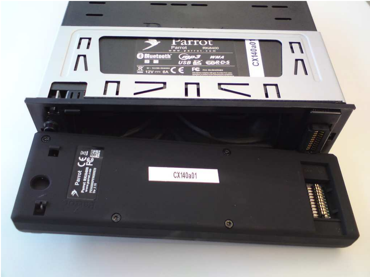
Photo: Front Panel with Radio unit - unmounted
