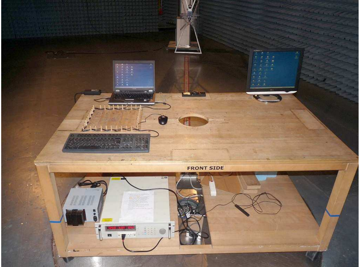
Test Setup Photo: radiated measurement
